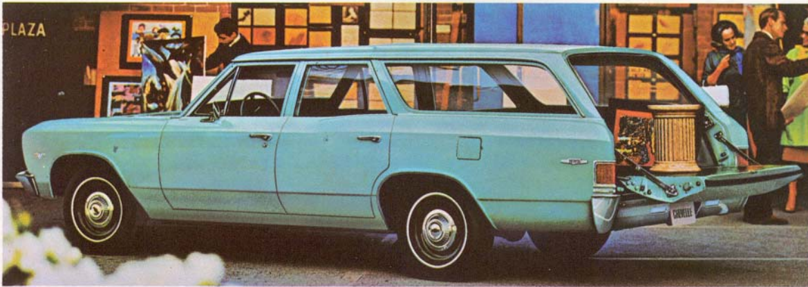
Malibu Station Wagon in Sierra Fawn. Rear opening is 54.6 inches wide by 28.5 inches high. Depending on model, standard power is the 140-hp Six or the 195-hp V8. Fully synchronized 3-Speed transmission is standard. 4-Speed fully synchronized transmission and Powerglide are available.
