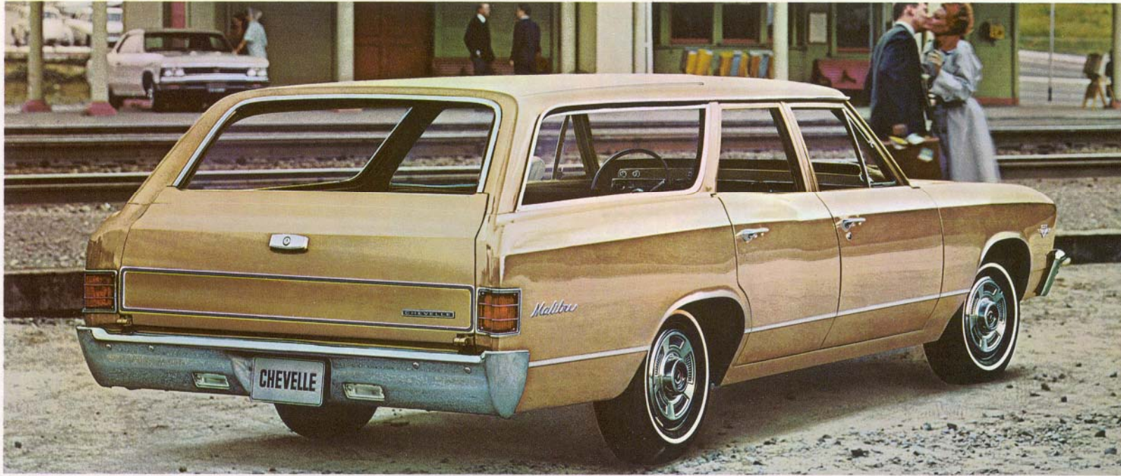
Malibu Station Wagon in Sierra Fawn. Rear opening is 54.6 inches wide by 28.5 inches high. Depending on model, standard power is the 140-hp Six or the 195-hp V8. Fully synchronized 3-Speed transmission is standard. 4-Speed fully synchronized transmission and Powerglide are available.
